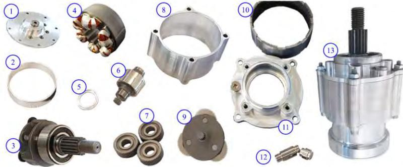
Cycloidal drive was designed. Functional prototype was built in rapid prototyping and tested.
