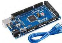
Arduino Mega for data collection from voltage and temperature sensors
