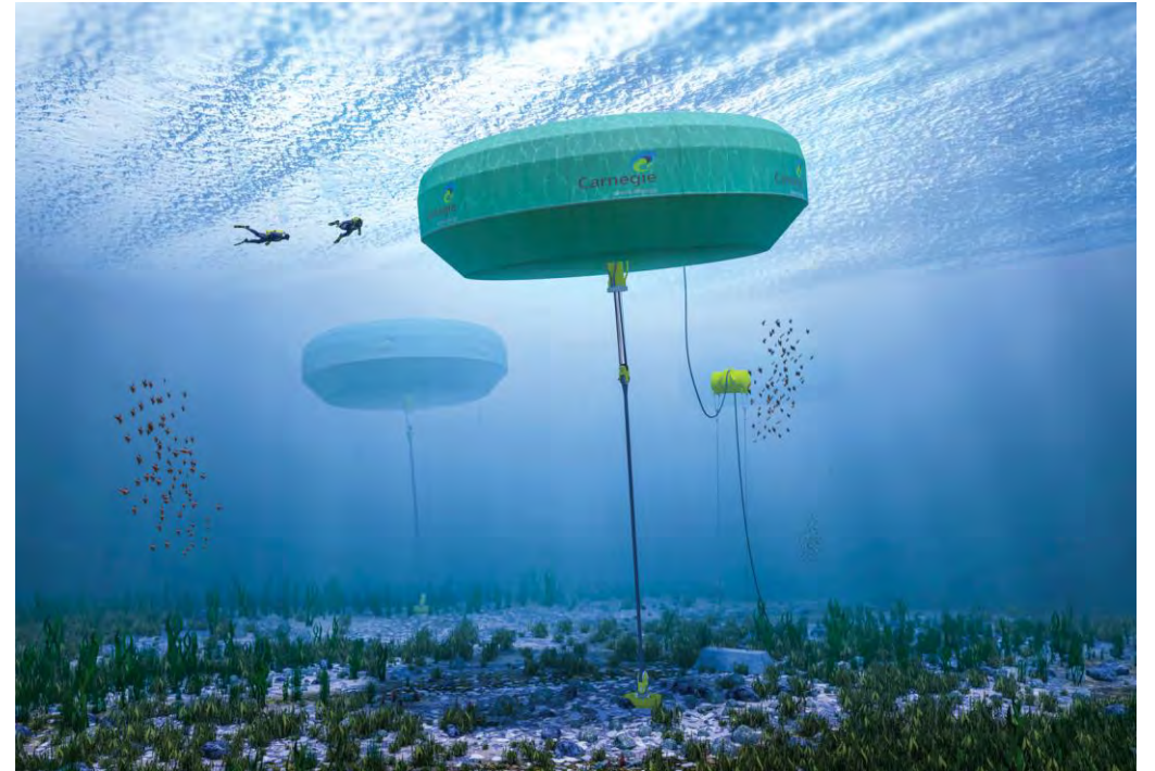
CETO is a fully submerged, point absorber developed by Carnegie
