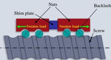
Tangential forces between spheres and grooves:
